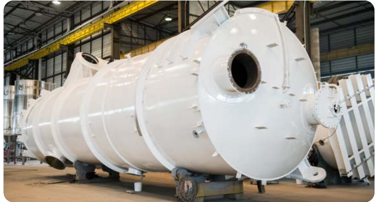
Brick-lined absorption tower
